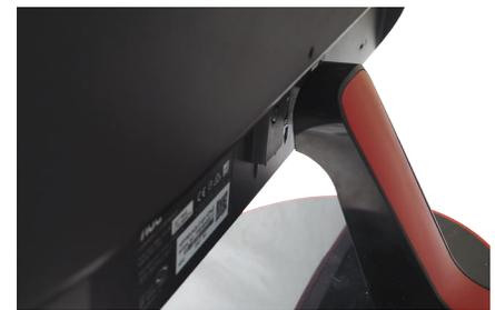
Before mouting this monitor, the stand needs to be removed first
